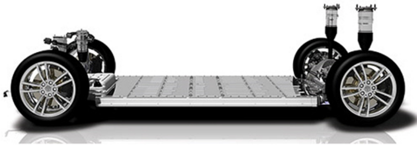
Figure 4: Battery in a Tesla S Model chassis. The 85kWh battery has 7,616 18650 cells in parallel/serial configuration. At $250 per kWh, the cost is lower than other Li-ion designs.
